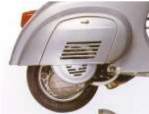
The larger engine hatch was fitted from late 1965 onwards
