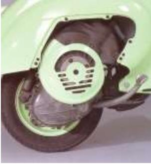
1963 spec with small hatch and body-coloured flywheel cover and wheels
